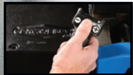
Class 3 safety hand-held remote controls bend, return and emergency stop functions.
