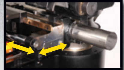
Programmable X2, Y2 axis pressure die movement.
