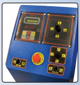
Programmable control of center roll.
